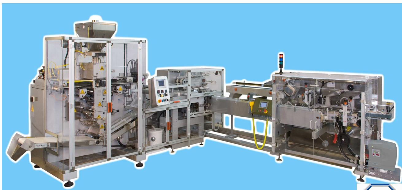
Complete MF line incorporating batching and cartoning system
